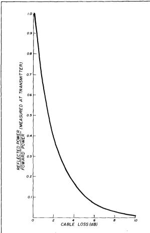
fig. 1. Ratio of reflected power to forward power as a function of cable loss (eq. 4).
